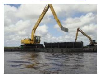
Several of the long reach excavators wereworking on the test plot at the conservancy on Oct 1, – at left is one of the excavators works on a timber mat to avoid becoming mired.
